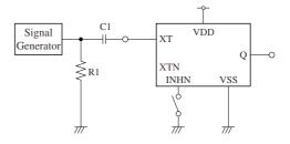
2Vp-p, 10MHz sine wave input signal C1:  $0.001 \mu F$  R1:  $50 \Omega$
