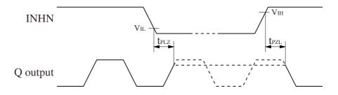
INHN input waveform  $tr = tf \le 10ns$
